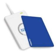
The NFC reader is a PC-linked contactless smart card reader/writer developed on the 13.56 MHz contactless technology. It is the world's first CCID-compliant contactless card reader/writer that follows both ISO 14443 and ISO 18092. This device is designed to support not only Mifare and ISO 14443 Type A and B cards but also FeliCa and NFC tags.
