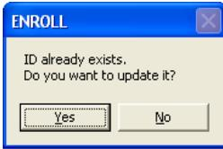
4. A user ID automatically increments from 1000. A fingerprint ID is automatically selected from 1 to 10, each corresponding to from the thumb of the right hand to the little finger of the left hand in an orderly manner. A user ID can be changed within the range of 1000~9999. If a user ID and a fingerprint ID are identical, a message “Do you want to update it?” will be pop up.
