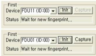
2. It uses from device list to select the device, click the “Init” button. It will be able to use HFDU04, HFDU06, HFDU08, HFDU11/14/06M/06S, MFDU03/13 and MFDU06. HFDU06, HFDU08 and HFDU11/14/06M/06S capture fingerprint by AutoOn. HFDU04, MFDU03/13 and MFDU06 must click “Capture” button.
