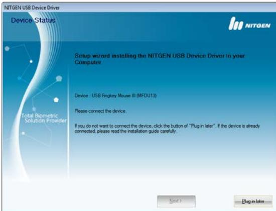
7. Connect the FRD to the USB port, and wait a moment. You can also click “Plug in later” to install it at a later time.
