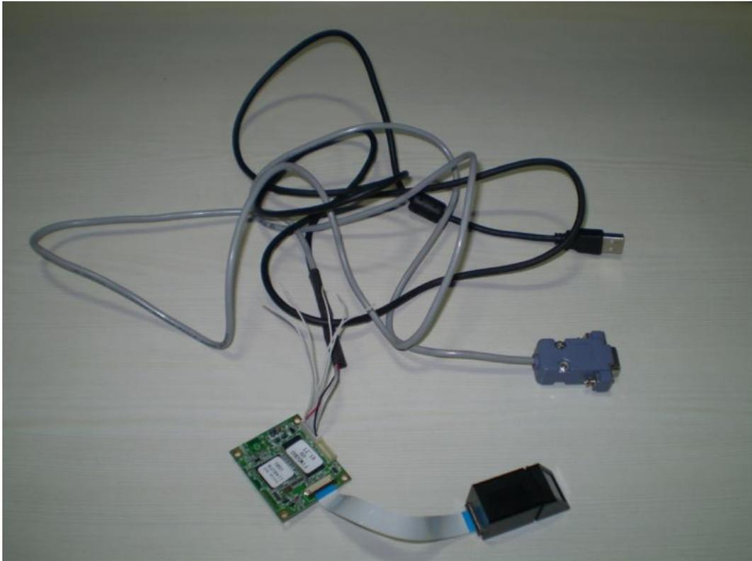
Connect the FIM module to computer as per above connections.
