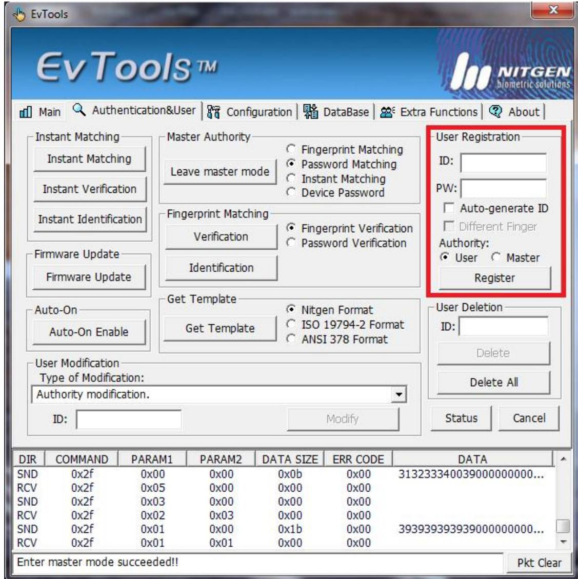
ii) Scanner will light up. Put Your finger on scanner for a moment,Following window will open.
