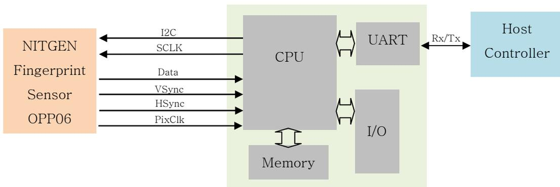
RS-232C communication data consist of 8-bit data, no parity, 1-bit start-bit and 1-bit stop-bit.
